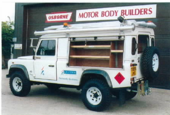
N/S view with shutter open, showing interior shelving and lift bar on shutter.
