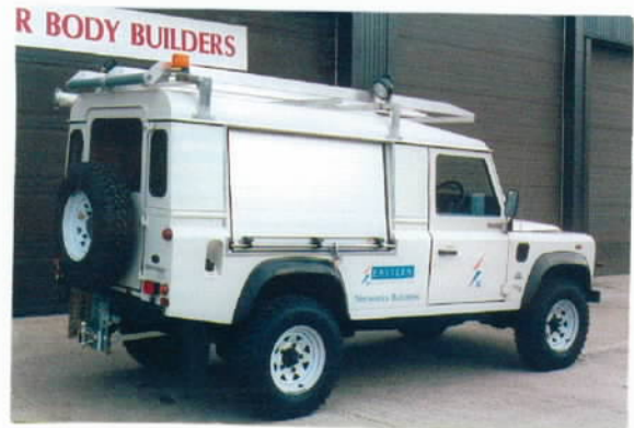
O/S view showing reduced length shutter, ladder rack, beacons and work lights.
