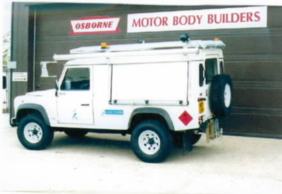
N/S view showing shutter, ladder rack, storage tube, beacons and work lights.
