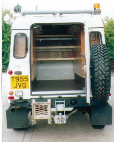
Rear view showing large access step, grab handle, towing facility, interior shelf assembly, roof rack rollers, floor overlay.
