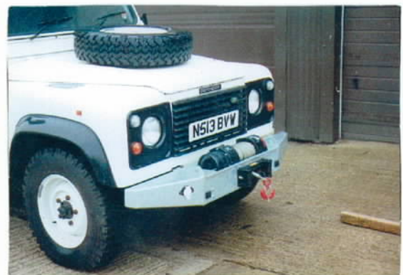
Front view showing 8000 lbs. line pull Ramsey winch, wanderlead control, fitted into galvanised steel mounting/bumper.
