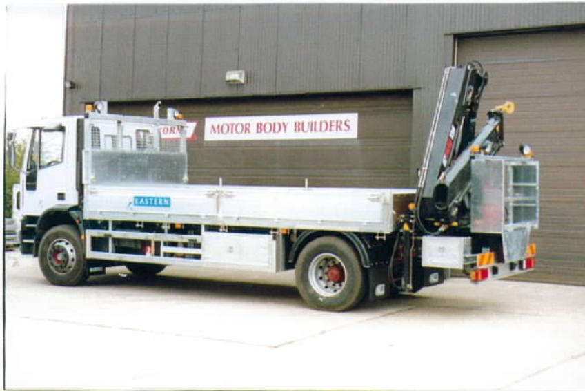
N/S view showing bodywork, skirt lockers, heavy duty headboard.
