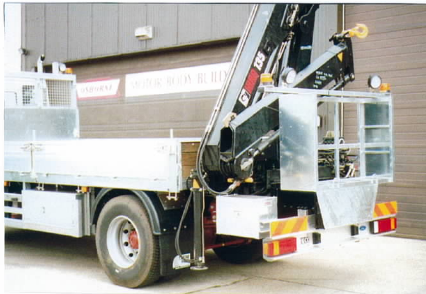
Rear view showing crane, timber baulk storage, skirt locker
